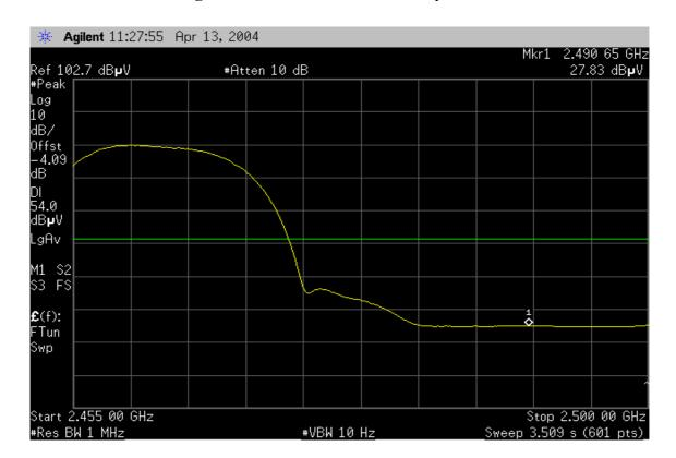
Detector mode: Peak Polarity: Horizontal
