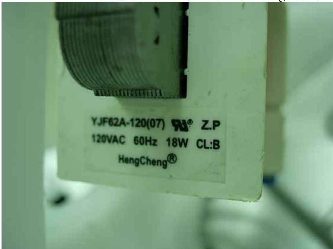
Photo 36 M/N: TSK-M3204MEQ, Label of Fan Motor
