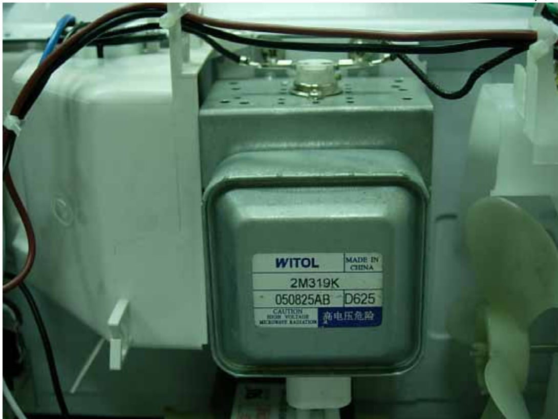
Photo 13 M/N: TSK-M3204ME, Magnetron
