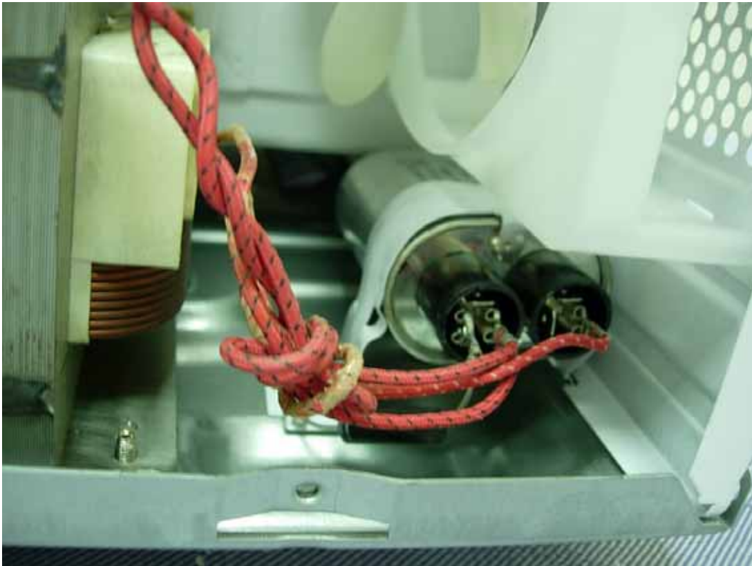
Photo 17 M/N: TSK-M3204ME, H.V. Capacitor
