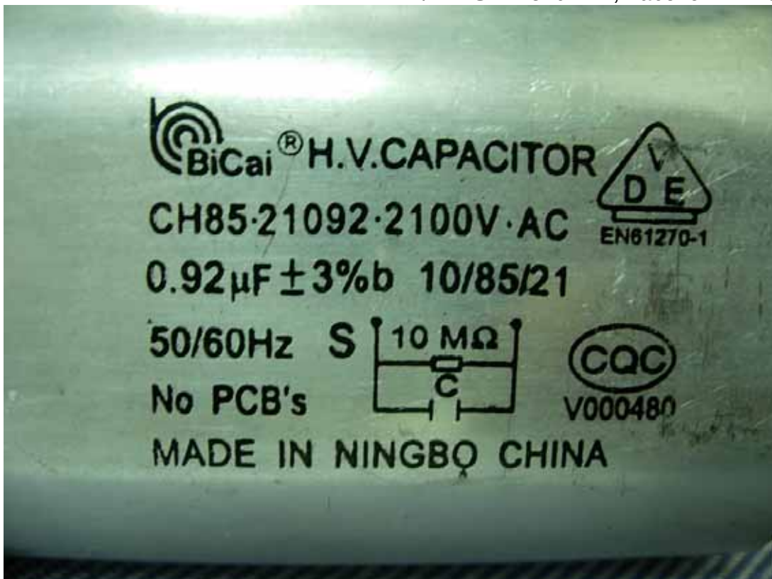
Photo 18 M/N: TSK-M3204ME, Label of H.V. Capacitor
