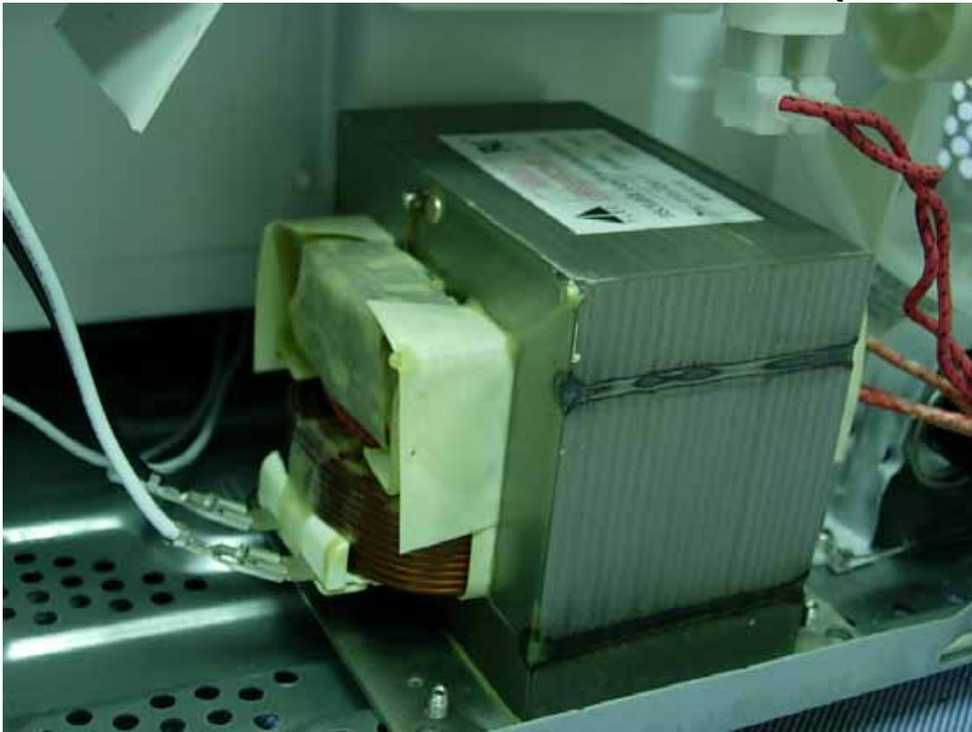
Photo 31 M/N: TSK-M3204MEQ, H.V. Transformer
