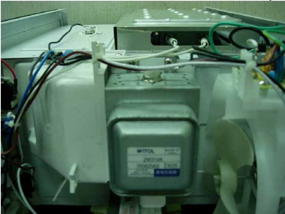
Photo 29 M/N: TSK-M3204MEQ, Magnetron
