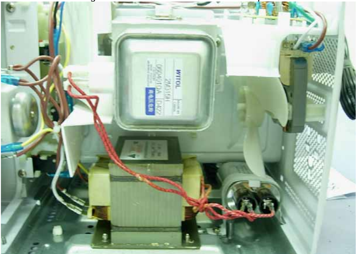
Photo 31 TSK-M1602MA/TSK-M1601MA Magnetron & H.V. Transformer & H.V. Capacitor & Fan Motor View
