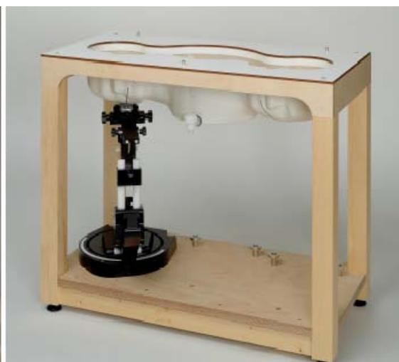
The DASY device holder has been made out of low-loss POM material having the following dielectric parameters: relative permittivity  $\epsilon=3$  and loss tangent  $\tan \delta=0.02$ . The amount of dielectric material has been reduced in the closest vicinity of the device, since measurements have suggested that the influence of the clamp on the test results could thus be lowered.
