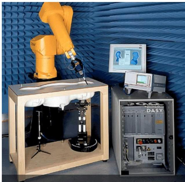
The system is based on a high precision robot (working range greater than 0.9m), which positions the probes with a positional repeatability of better than  $\pm 0.02\text{mm}$ . Special E- and H-field probes have been developed for measurements close to material discontinuity, the sensors of which are directly loaded with a Schottky diode and connected via highly resistive lines to the data acquisition unit.
