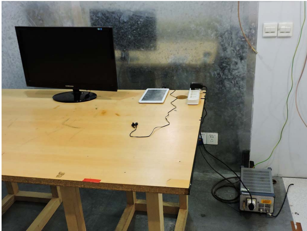
Conducted Emission Test Setup:
