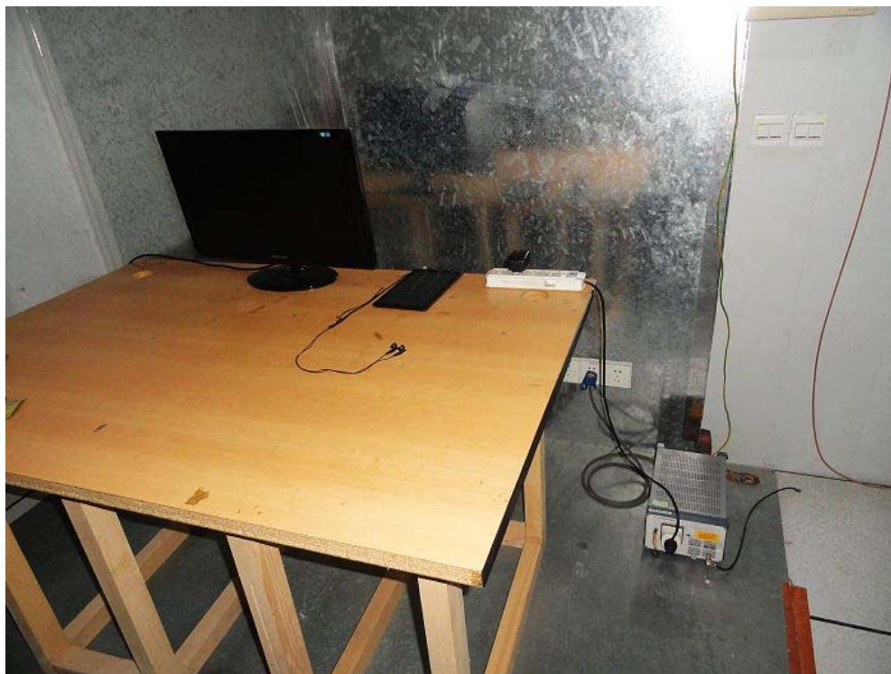
Conducted Emission Test Setup:
