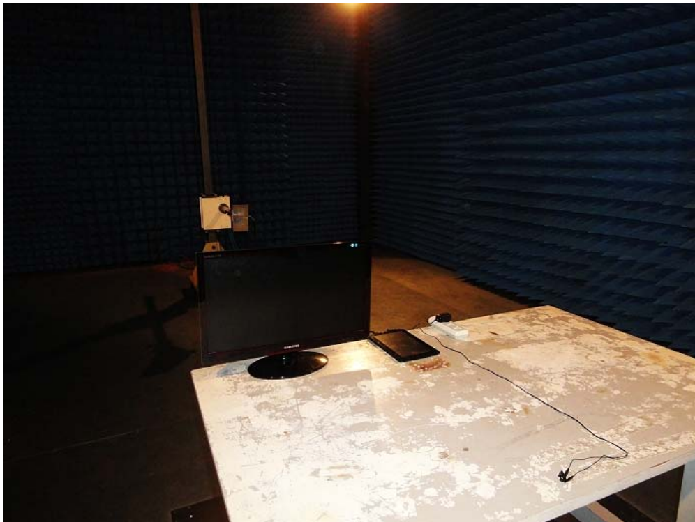
Radiated Emission Test Setup:
