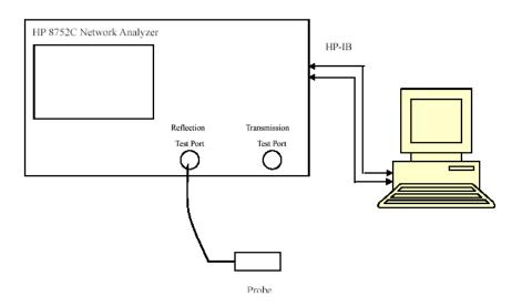
Liquid Verification Setup Block Diagram
