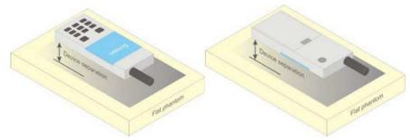
Figure 5 - Test positions for body-worn devices
