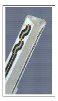
Inside view of EX3DV4 E-field Probe
