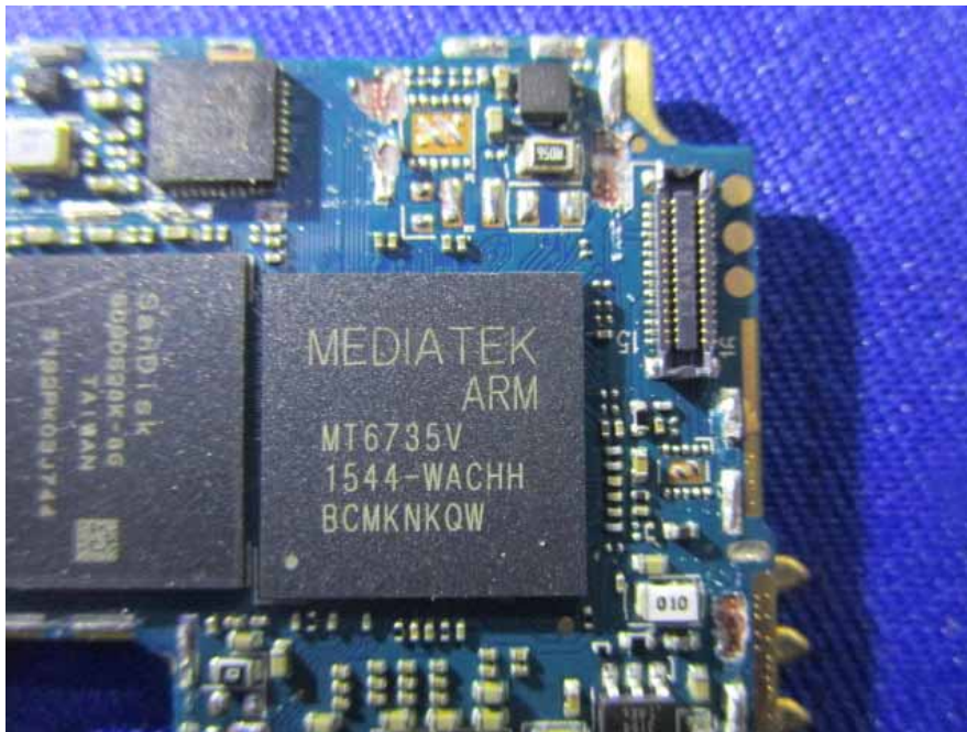
EUT –Main Chip View
