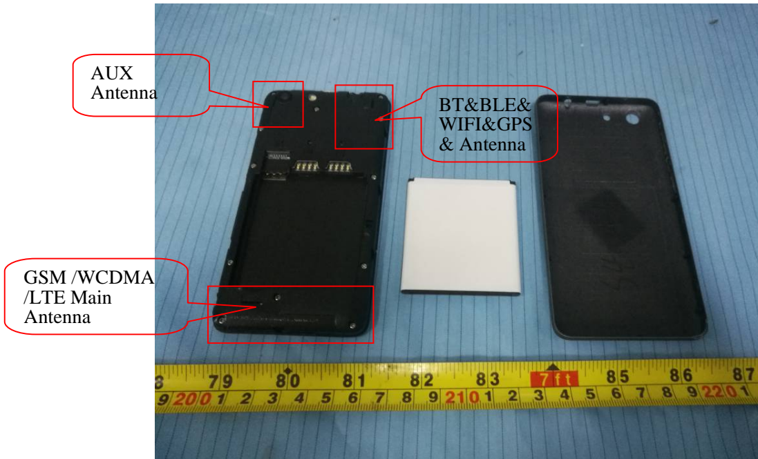
EUT – Cover off View 1
