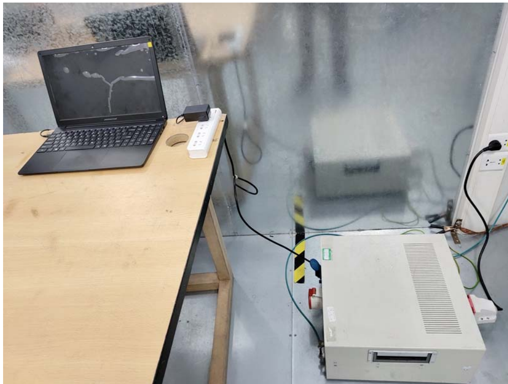
Conducted Emission Test Setup:
