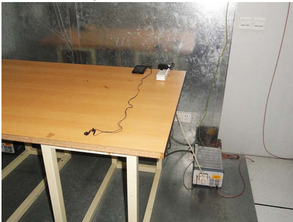
Conducted Emission Test Setup:
