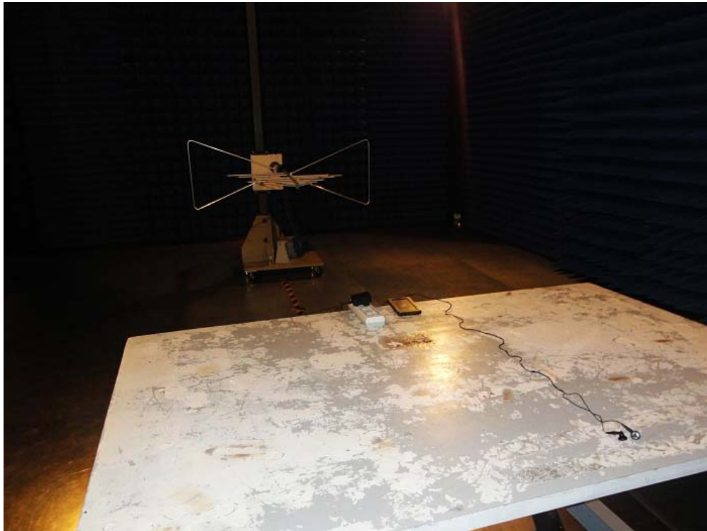
Radiated Emission Test Setup:
