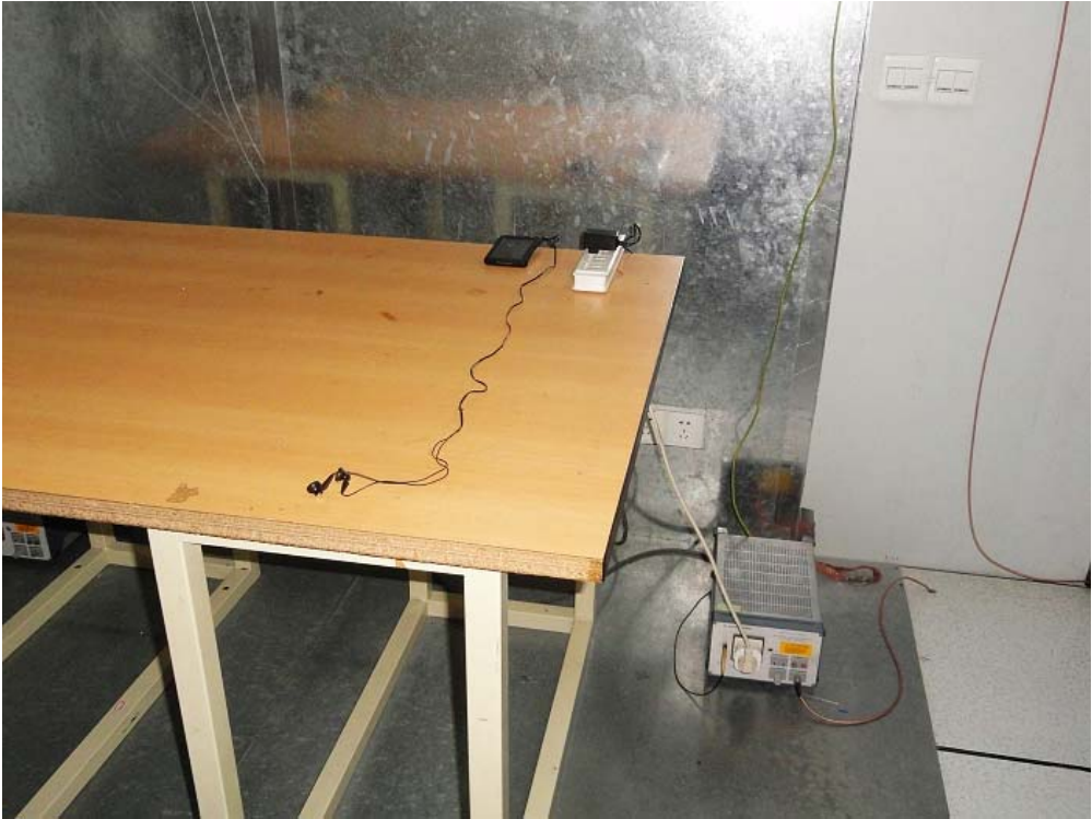
Conducted Emission Test Setup:
