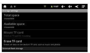
Micro SD Card: View the total capacity of Micro SD card, Micro SD card free space, uninstall Micro SD card, and format the data on the Micro SD card memory, built-in Flash Memory: Built-in Flash memory available view space. Device memory: View device memory free space.
