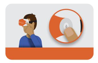
To conserve power, the screen will turn off when not in use. It is activated by a sensor inside the headset.
