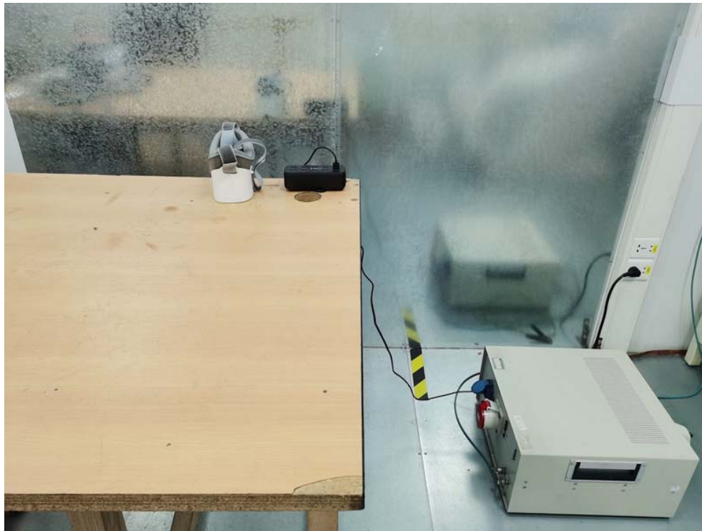
Conducted Emission Test Setup:
