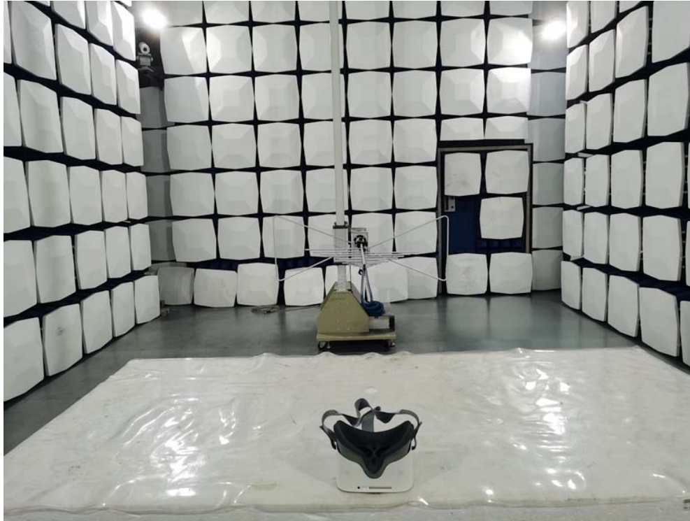
Radiated Emission Test Setup:
