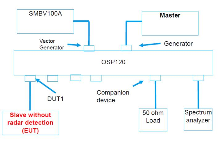
The UUT is a U-NII Device operating in Client mode without radar detection. The radar test signals are injected into the Master Device.
