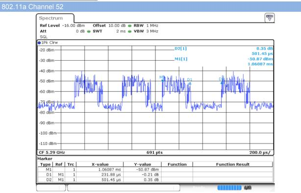
The channel loading Specification of Ton/ (Ton +Toff) as the file streaming between master to client is 87.4%.
