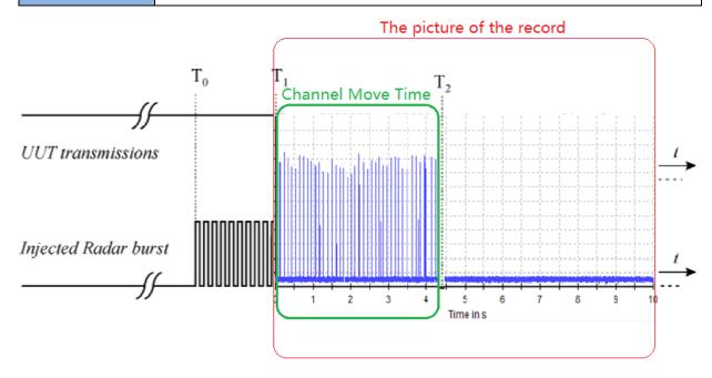
T0 denotes DFS test signal start generated on the channel.
