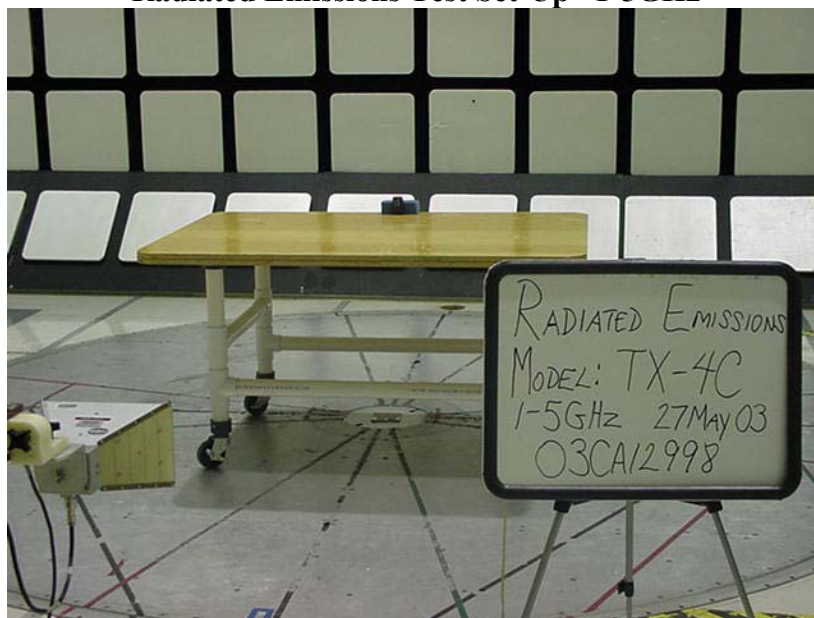
Radiated Emissions Test Set-Up –1-5GHz
