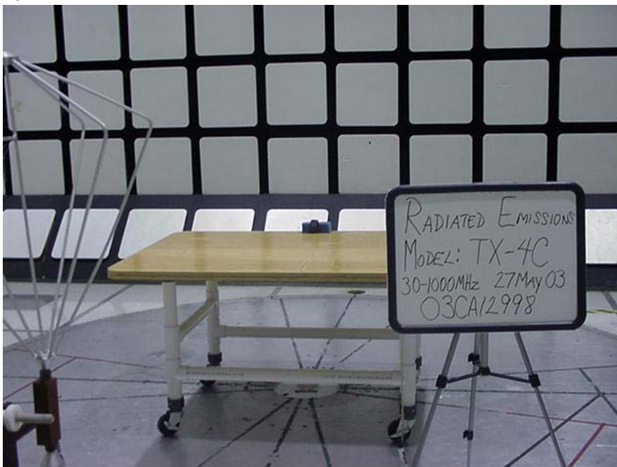
Radiated Emissions Test Set-Up – 30-1000MHz
