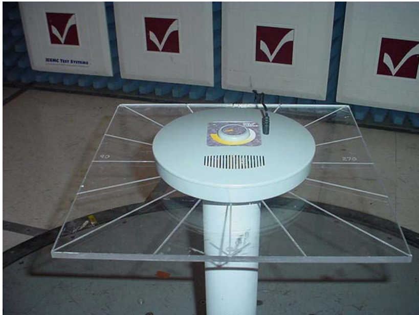
View of the EUT during Radiated Emission Testing in the 3 Meter FCC Listed Chamber
