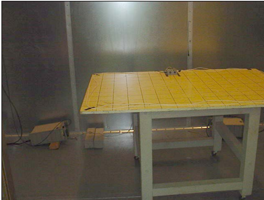
View of the EUT during Conducted Emission Testing in the 3 Meter FCC Listed Chamber
