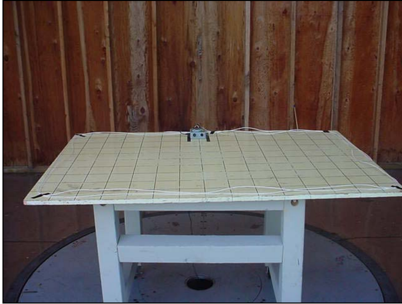
View of the EUT during Radiated Emission Testing on the 10 Meter OATS
