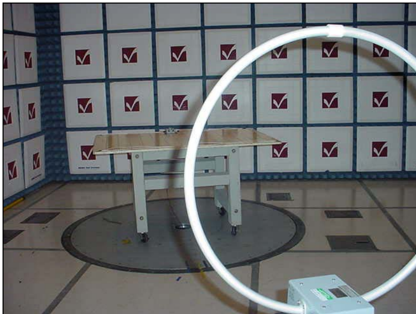
View of the EUT during Radiated Emission Investigative Testing In the 3 Meter Chamber
