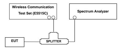
(Configuration of conducted Emission measurement)
