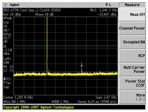
■ Secondary EVDO MODE (684 CH.) Conducted Spurious Emissions - 2
