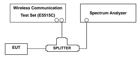
(Configuration of conducted Emission measurement)
