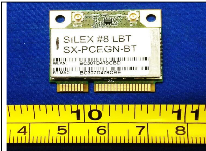
Radio Board – Top View with Shielding
