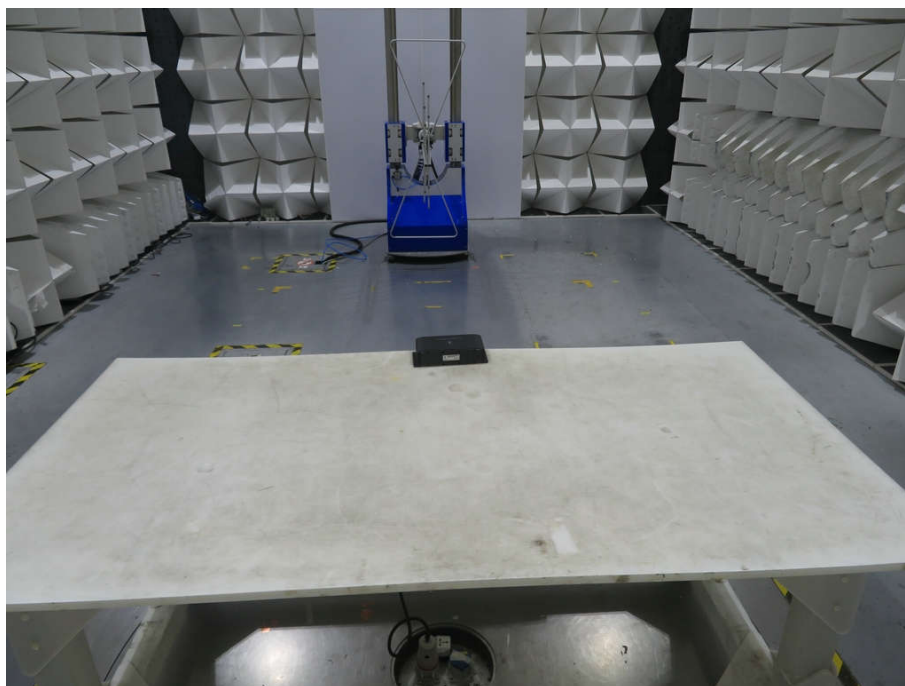
Radiated spurious emission Test Setup-1(Below 1GHz)
