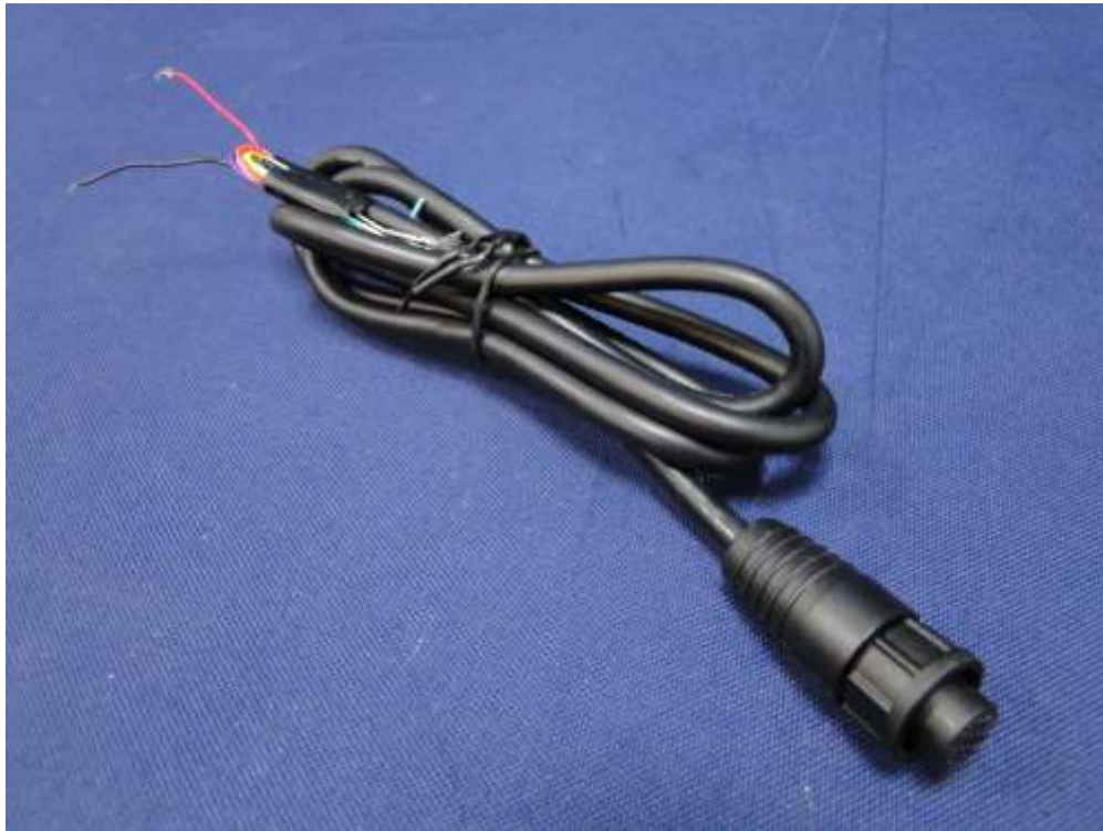
(7) EUT Photo _ 12pin Power & data Cable
