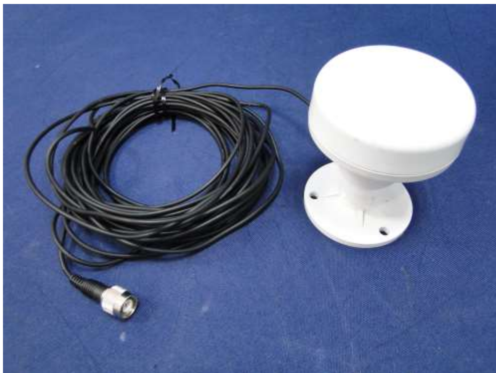
(8) EUT Photo _ GPS antenna with 10m Cable
