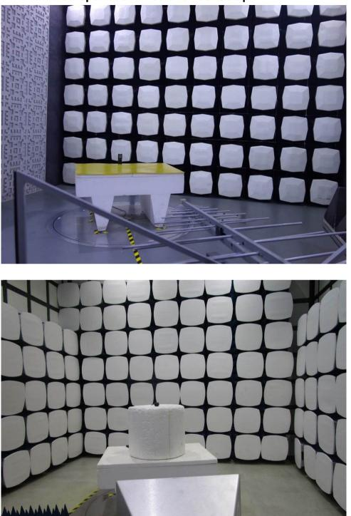
**1.2** Radiated Spurious Emissions Test Setup
