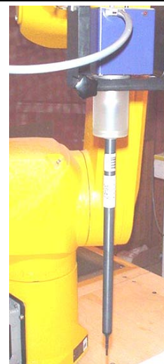
EX3DV4 E-Field Probe
