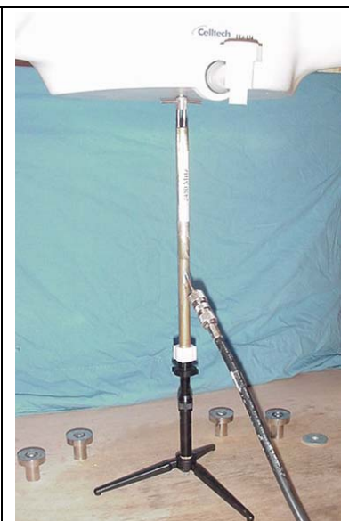
2450 MHz Validation Dipole Setup
