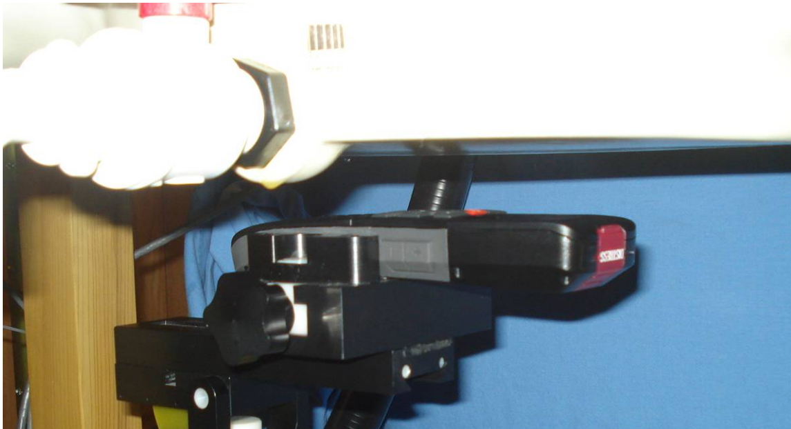
DUT front (screen side) facing phantom - 25mm spacing
