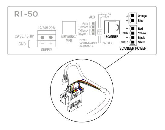
If you ever need to replace or refit the 8-pin RJ45 connector on the interconnection cable, use a RJ45 crimping tool and wire as follows:
