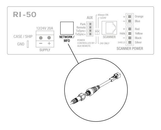
The RI-50 can be connected directly to any Simrad<sup>®</sup>-compatible multi-function display or to a network switch such as an NEP-2.
