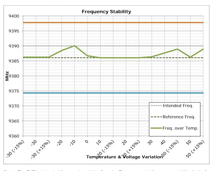
**Note:** The EUT is intended for use also within Canada. The more strict frequency stability limit of 800 ppm from RSS-238 has been applied to the data.
