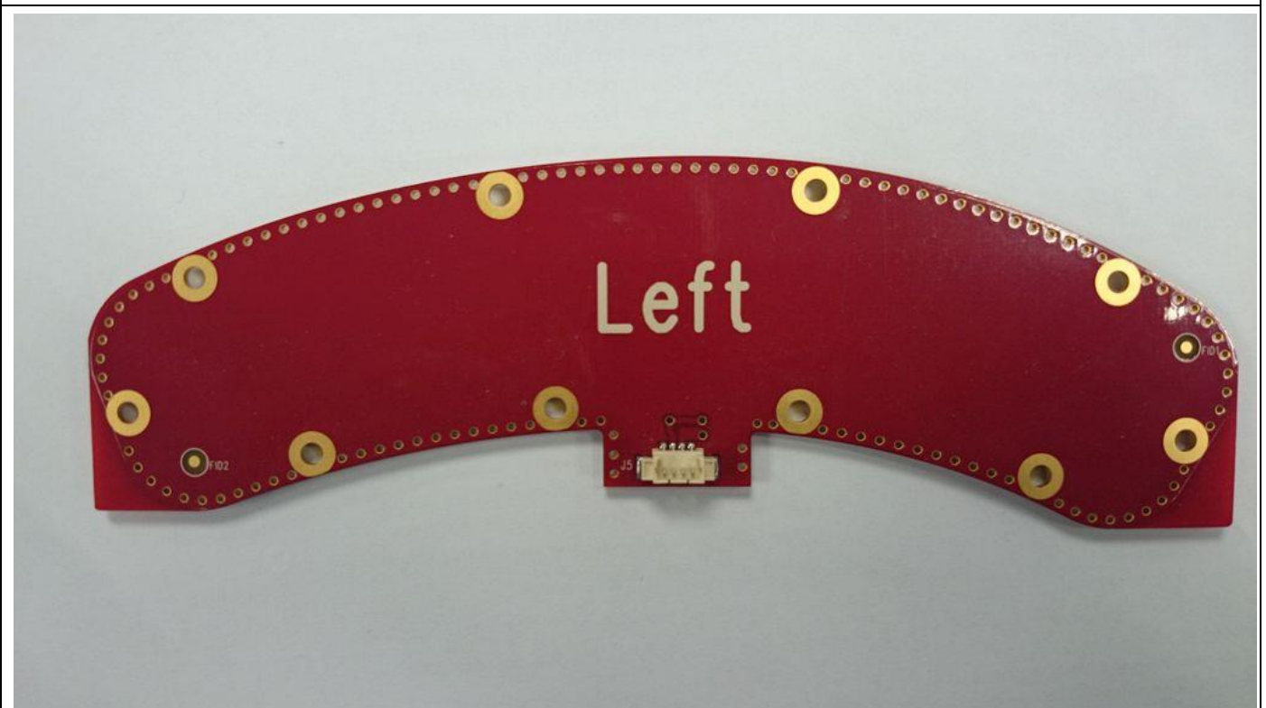
HALO LED PCBA – LEFT & RIGHT (LEFT SHOWN)
