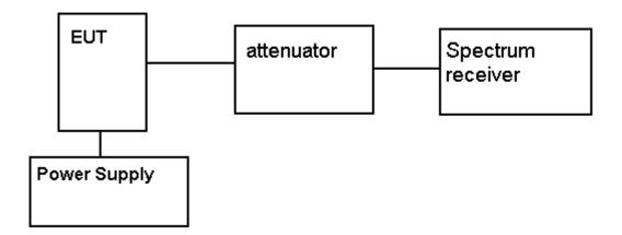
**METHOD OF MEASUREMENT:** The procedure used was TIA/EIA-603-C:2004
