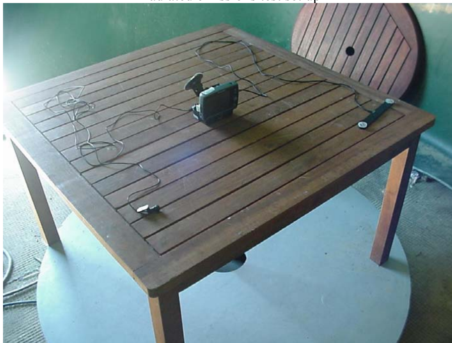
Radiated emissions test set up
