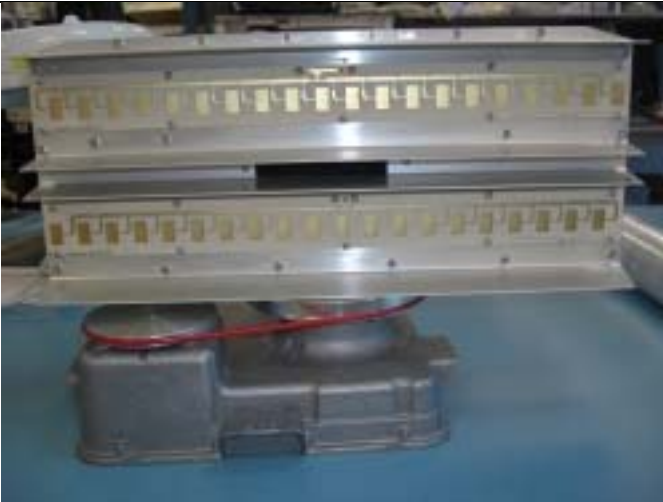
Internal main assembly – motor & rotary joint
