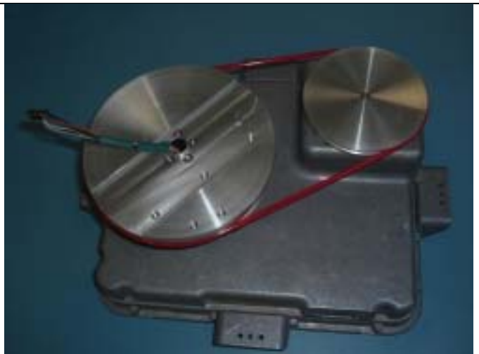
Internal main assembly – drive belt and pulleys
