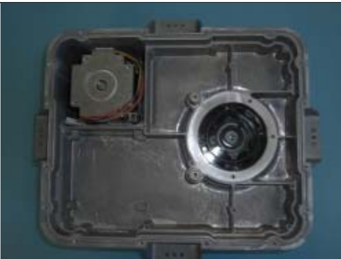
Internal main assembly – motor & rotary joint
