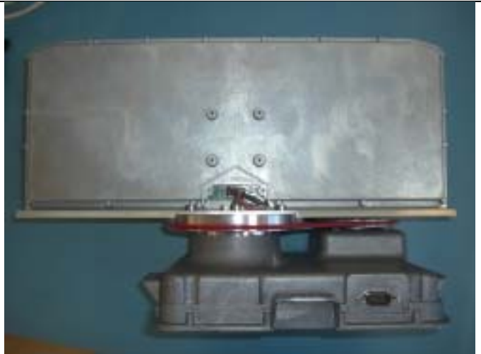
Internal main assembly – drive belt and pulleys
