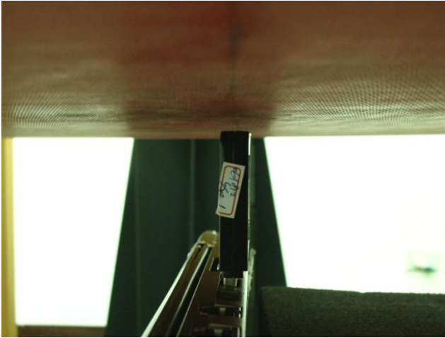
Direct Laptop Plug-in for Tip Mode (Tip Mode with Phantom 5 mm Gap)
