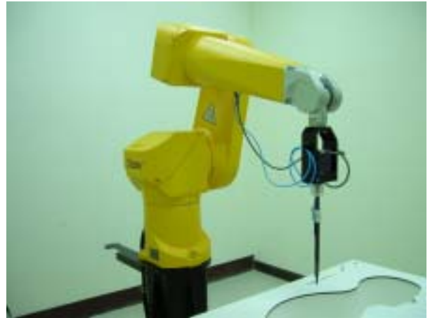
Fig. 5.2 Probe setup on robot
