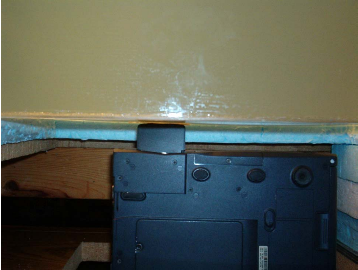
Fig. 3. Photograph of the Dell Model PP01L Host Computer at 90° with the edge of the Arcadyan EZ-Stream Universal Wireless Cardbus Adapter pressed against the bottom of the planar phantom. This is Configuration 2 for SAR testing and represents the case of a bystander at a distance of 0 cm from the edge of the Cardbus Adapter.
