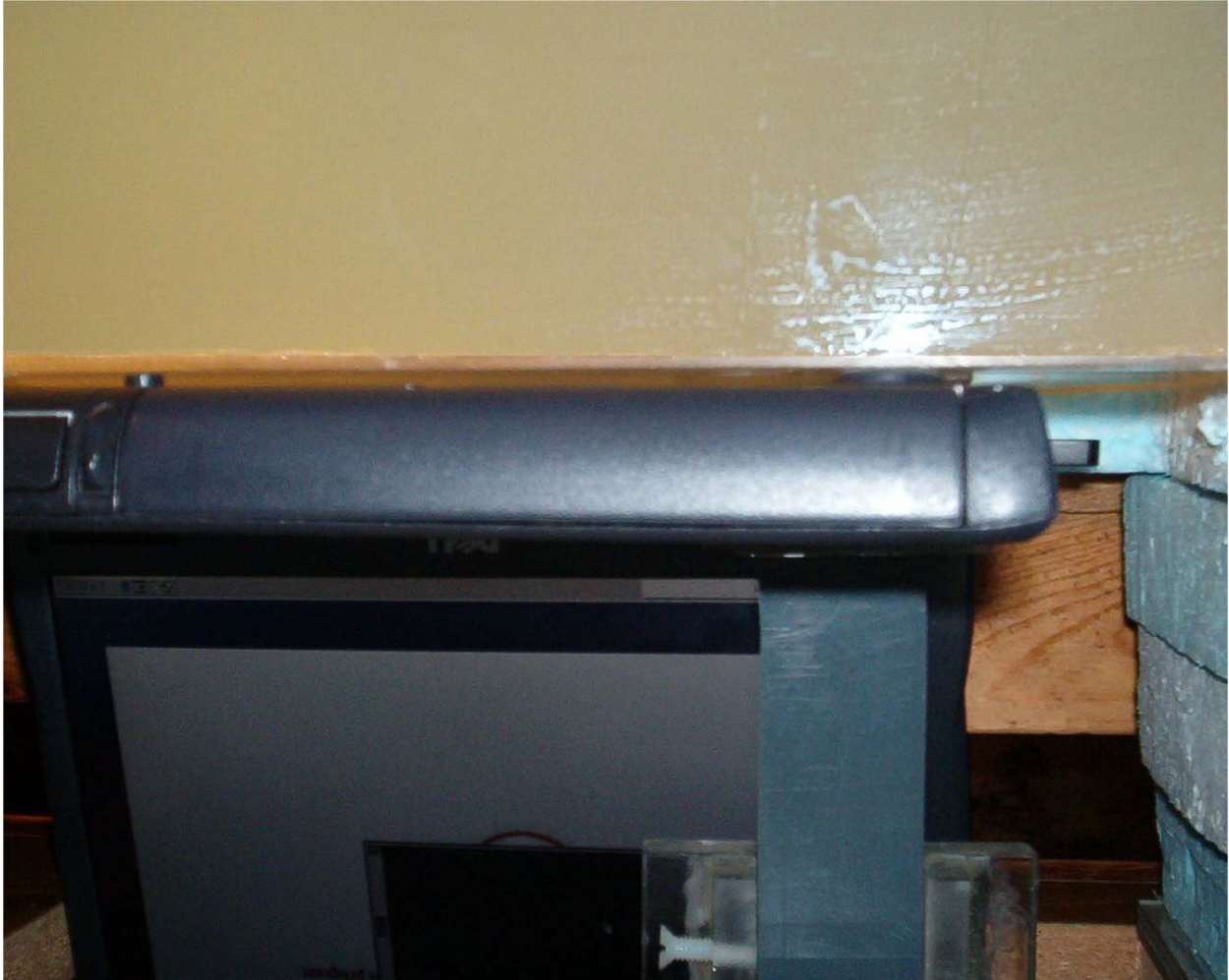
Fig. 2. Photograph of the bottom of the Dell Model PP01L Host Computer with Arcadyan EZ-Stream Universal Wireless Cardbus Adapter pressed against the bottom of the planar phantom. This Configuration 1 – Laptop position for SAR testing.
