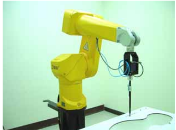
Fig. 5.2 Probe setup on robot
