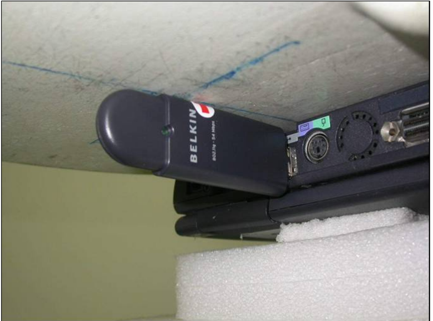
The edge of the EUT to the flat phantom distance 0 mm
