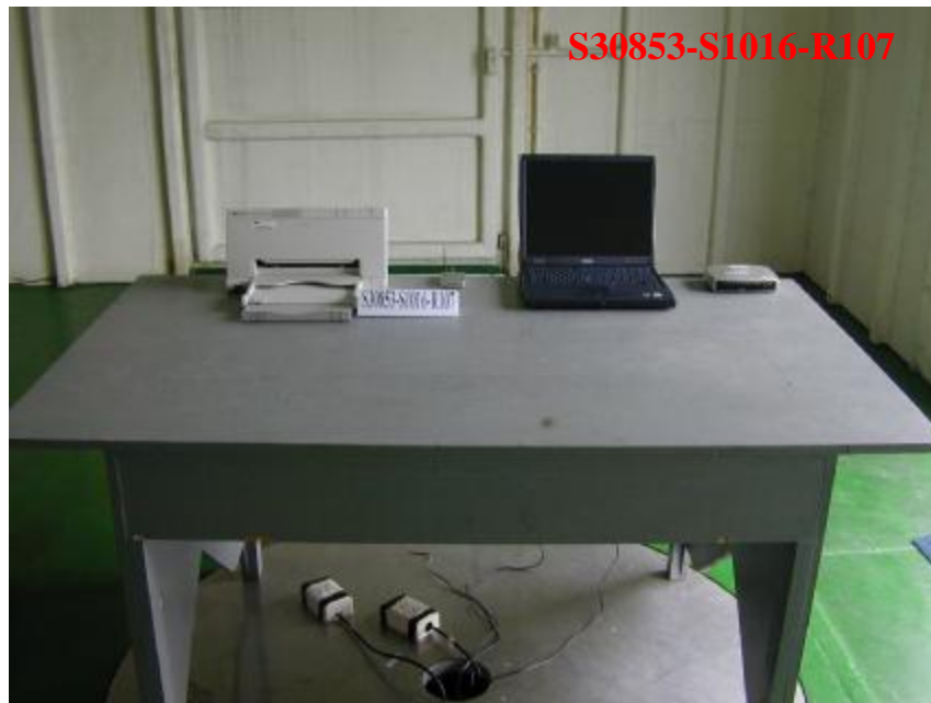
Photo 2: Radiated Emission Test Set-up
