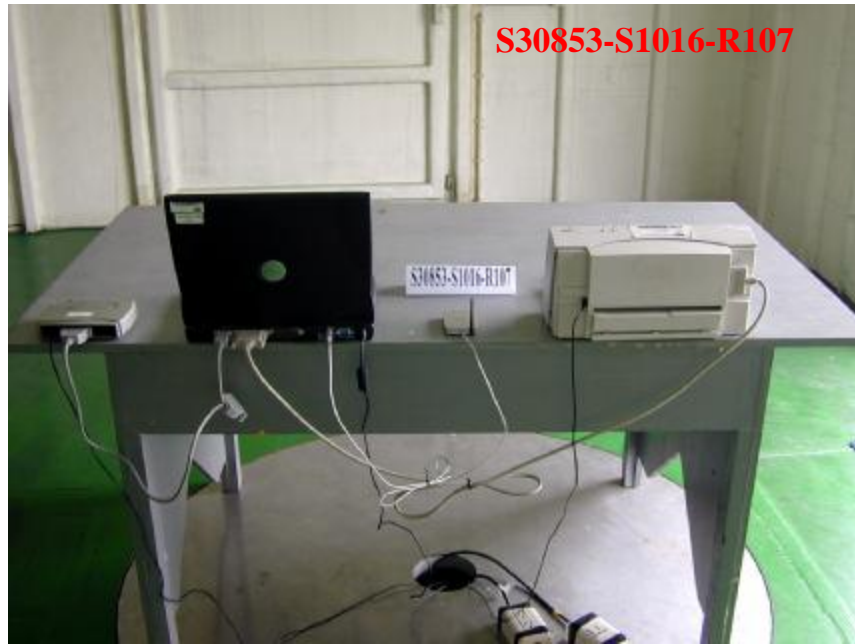
Photo 3: Radiated Emission Test Set-up
