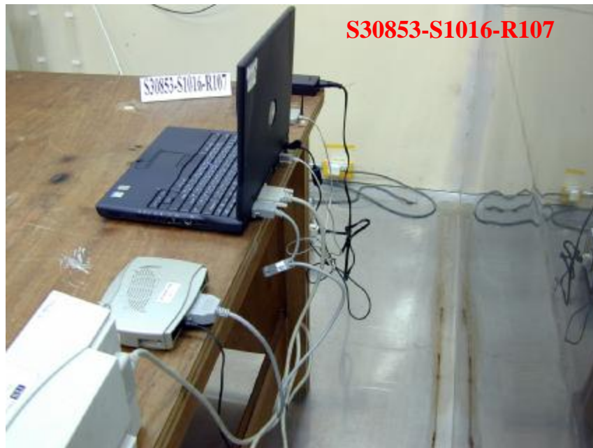
Photo 3: Conducted Emission Test Set-up
