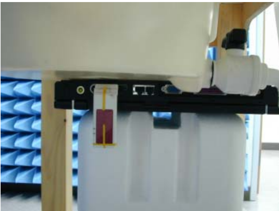
Fig.8 Photograph of the Bottom of the Pc is paralleled and at a distance of 0.0 cm from the base of the phantom, but 0.6 cm Spacing between
