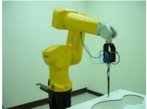
Fig. 5.2 Probe setup on robot
