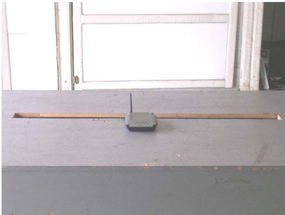
Photo 1: Radiated Emission Test Set-up
