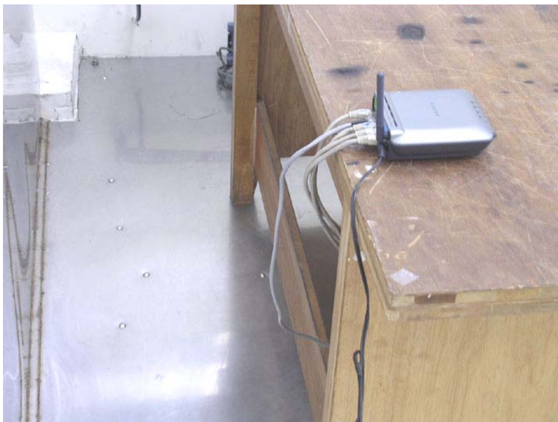
Photo 2: Conducted Emission Test Set-up
