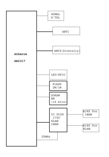
3.3V 1.8V AR2317 480mA SDRAM 100mA FLASH 30mA IP175C 547mA 670mA 547mA TOTAL CURRENT TOTAL POWER 0.98W 2.21W
