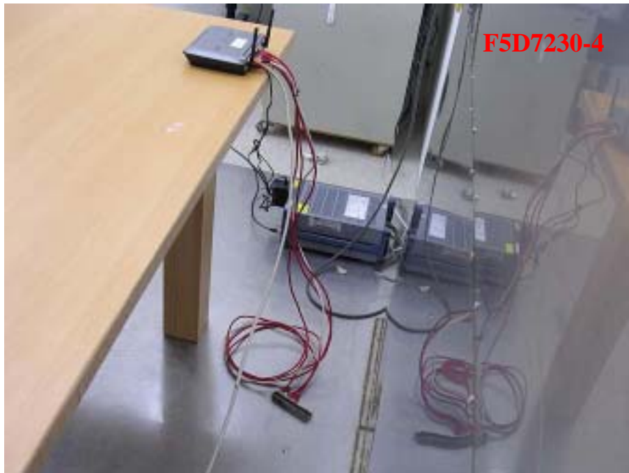
Photo 2: Conducted Emission Test Set-up
