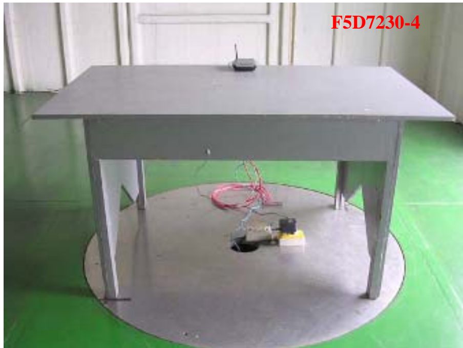
Photo 2: Radiated Emission Test Set-up
