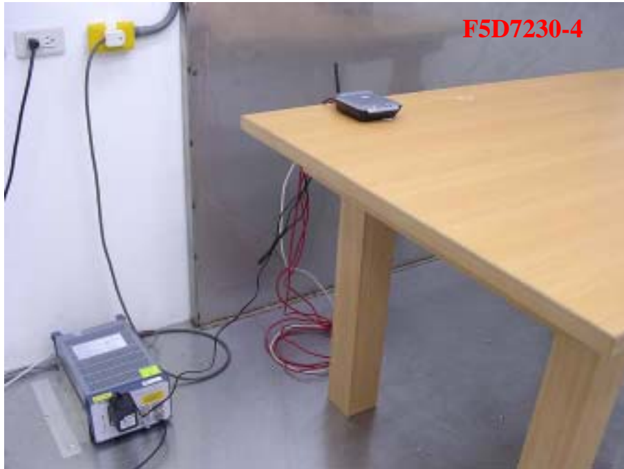
Photo 2: Conducted Emission Test Set-up
