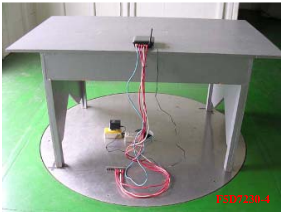
Photo 2: Radiated Emission Test Set-up
