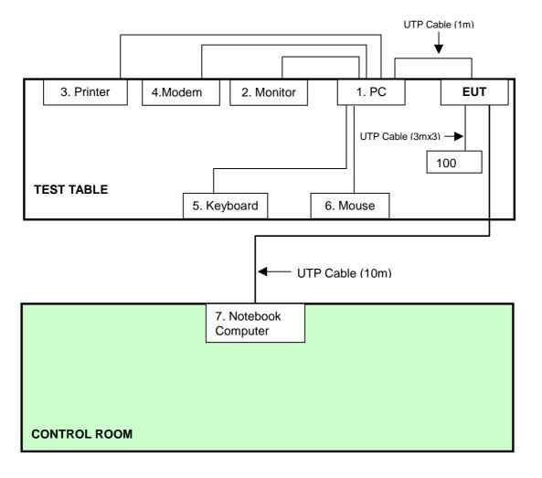
**NOTE:** 1. Support unit 7 was kept in the control room during the test.
