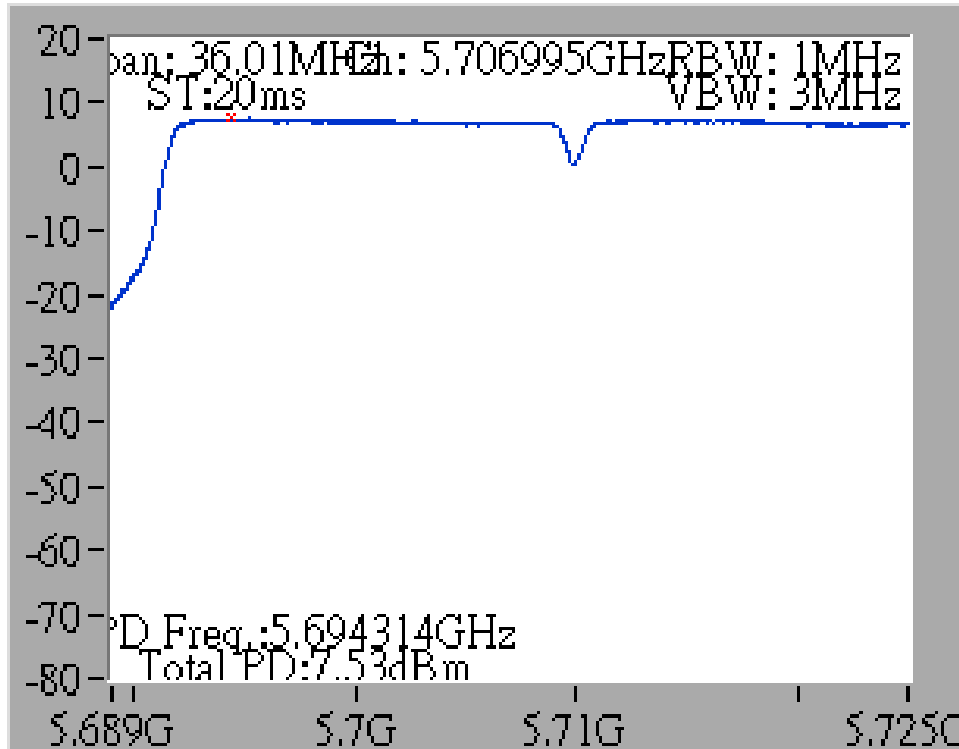
Power Density Plot on Configuration IEEE 802.11ac MCS0/Nss1 VHT40 / Chain 1 + Chain 2 + Chain 3 + Chain 4 / 5710 MHz (UNII 3)
