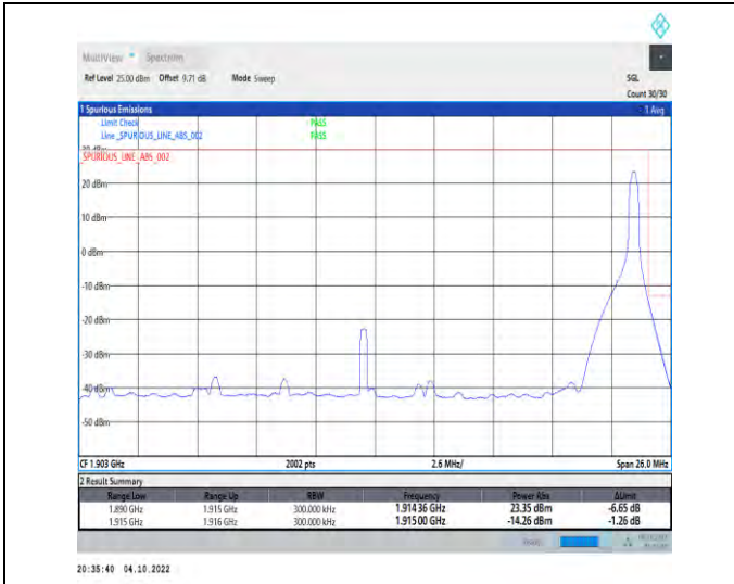
1-N25-PC3-15-25-H-2-DFT-QPSK-Edge_1RB_Right-1 @132-Ant1-1-seegraph-PASS-see graph
