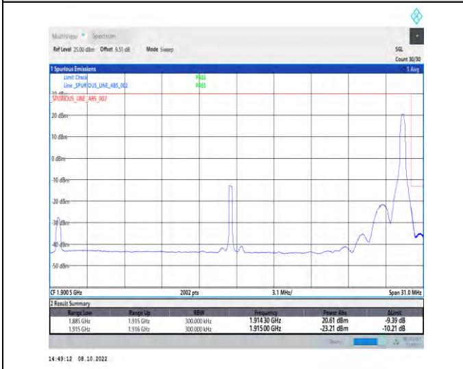
1-N25-PC3-15-30-H-5-CP-QPSK-Edge_1RB_Right-1 @159-Ant1-1-seegraph-PASS-see graph
