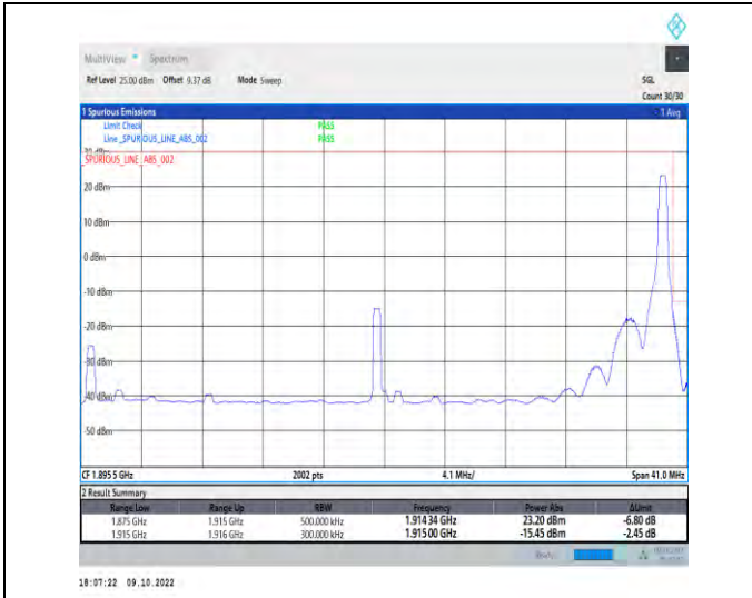
1-N25-PC3-15-40-H-2-DFT-QPSK-Edge_1RB_Right-1 @215-Ant1-1-seegraph-PASS-see graph
