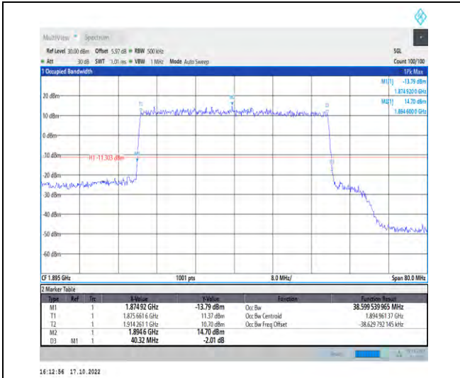
1-N25-PC3-15-40-H-1-DFT-QPSK-Outer_Full-216@ 0-Ant1-38.6-40.320-≤40-PASS
